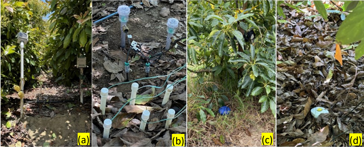
Fig. 3. Various soil moisture sensors used in California avocado orchards (Acclima, Watermark, and tensiometer soil moisture sensors and telemetry devices (a & b), CropX soil moisture probe (c), and Metergroup Teros 54 soil moisture probe (d)).
